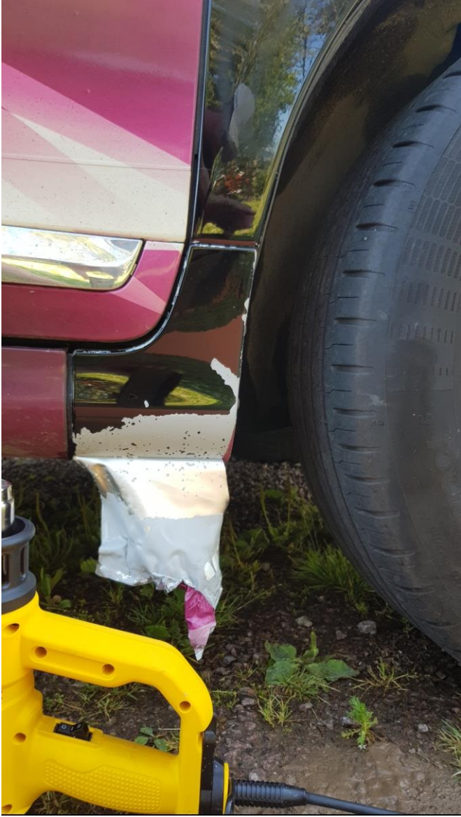
Figure 6. More Illuminite delamination
