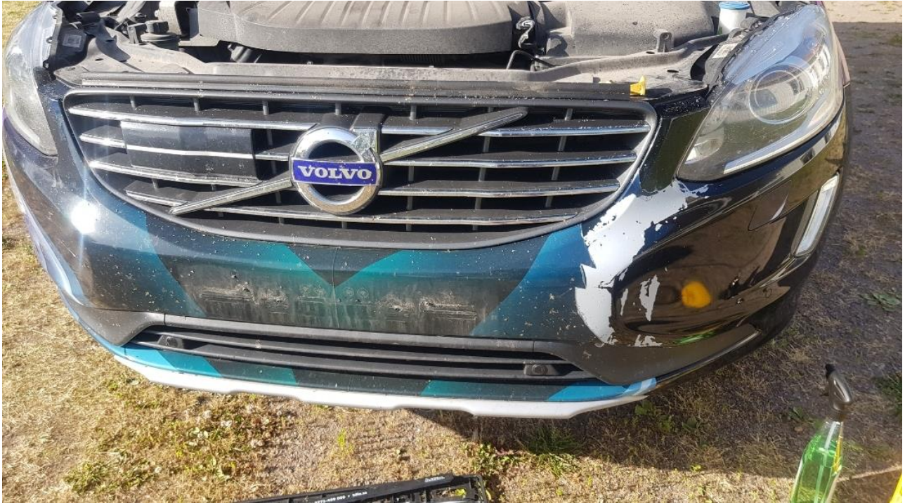
Figure 4. Front hood showed some delamination on front edges
