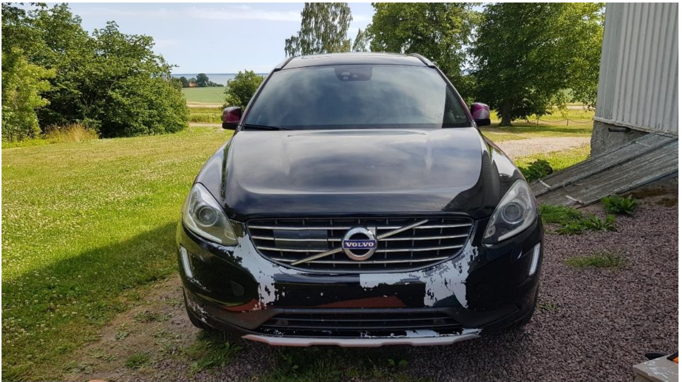
Figure 5. Bumper with Illuminite adhesive
