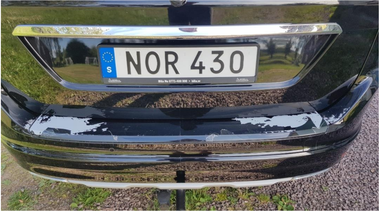
Figure 2. Adhesive on the flat side of the back bumper.
