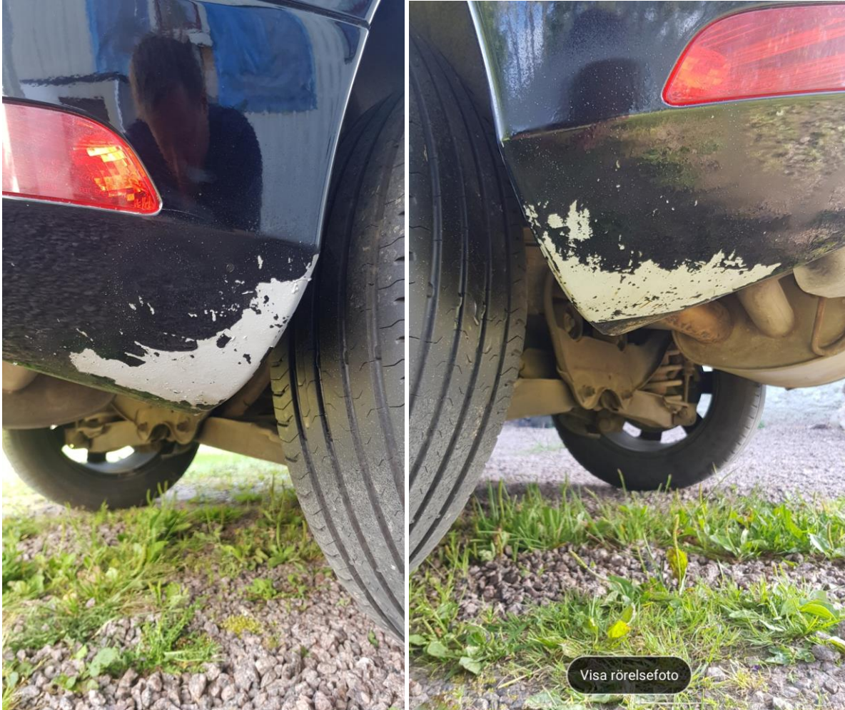
Figure 1. Adhesive on each side of the bottom section of back bumpers.
